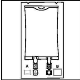
The integrity indicator (Oxalert™) **A** should be inspected before removing the overwrap. If the indicator is black the overwrap is damaged and the product should be discarded.
